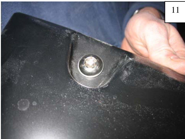
Insert one Screw/Washer assembly through each pocket hole drilled in Step 9.
