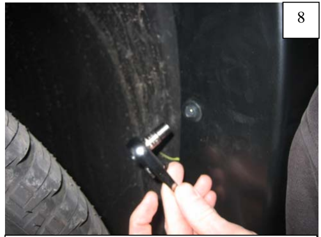
Holding flare in position on fender, reinstall factory screws removed in Step 5.
