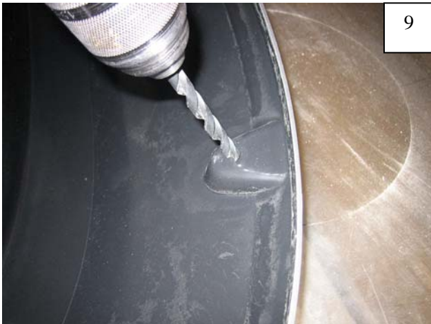
Prior to paint, use a drill with 5/16" bit to drill holes at indents in pockets (10 places). Drill from inside of parts.
