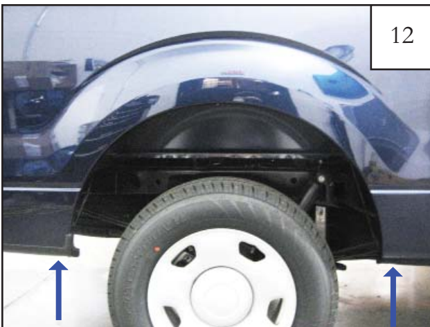
Remove two factory bolts with a 10 mm socket wrench.
