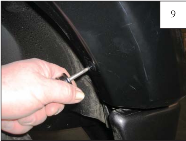
Still holding flare to fender, install tuflocks using a Phillips screw driver. See step 10.
