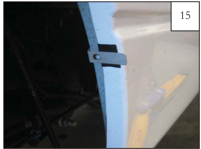
Install a long clip over each of the four black tabs placed on the sheet metal in Step 14.
