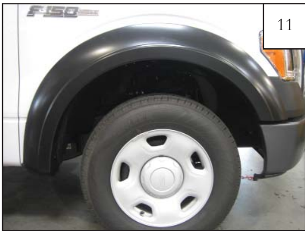
Completed front flare installation.
