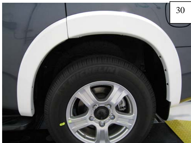
Once all screws have been started, apply pressure towards vehicle at each fastening point as you tighten all screws.
