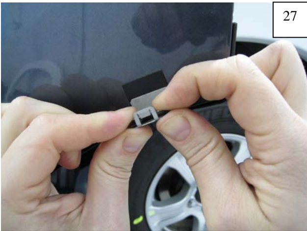
Snap each clip shut once aligned.
