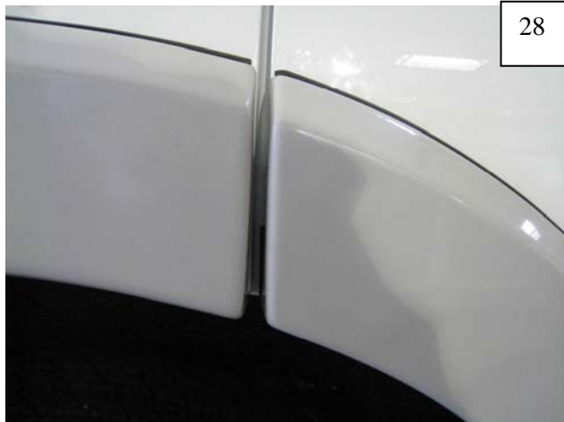
Position Door Piece on fender, aligning with edge of sheet metal along door, but not extending into the door seam.
