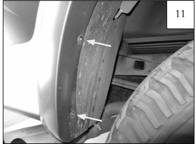
Use a 7/32 socket to remove the 2 factory screws located at the rear of the wheel well. Retain screws for re-installation later.
