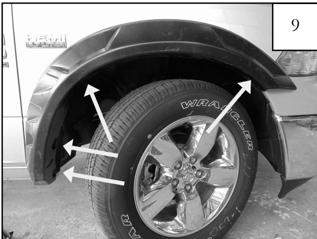
Reinstall 4 screws with an 8mm socket that were removed in Step 1. Press firmly on flare and tighten all screws.
